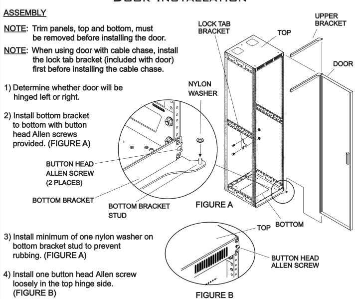
5) Install door onto bottom bracket stud, and holding door, install upper bracket stud to top of door. (FIGURE A) As an assembly, slip the upper bracket, with door attached, under the head of the loose screw on the top hinge side. Now install the second screw in the upper bracket and tighten both screws.
